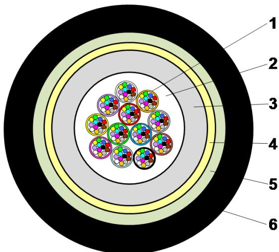
1. "Compact tube" : 6 or 12 single-mode or multi-mode optical fibers 50/125 assembled under "peelable" thermoplastic skin
