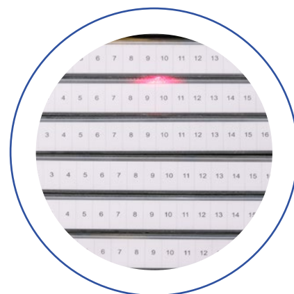
Quick identification with the use of a VFL, thanks to the clear front shutter
