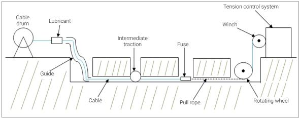
Figure : example showing the installation of optical cable in an underground duct.
