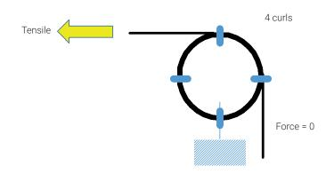
Ideally, these loops should be made as close to the anchoring clamp. It is however possible to lock them between the anchoring point and the entrance of the box.
